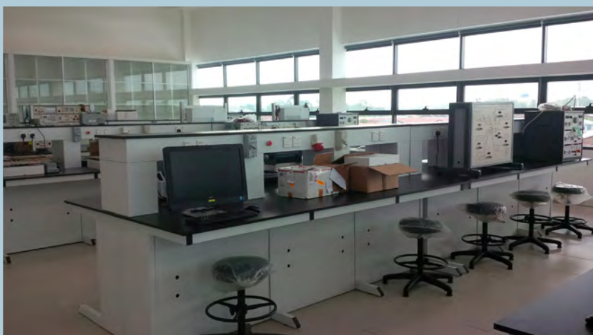
Island bench with reagent rack for extra working space and mounting of electrical power points
