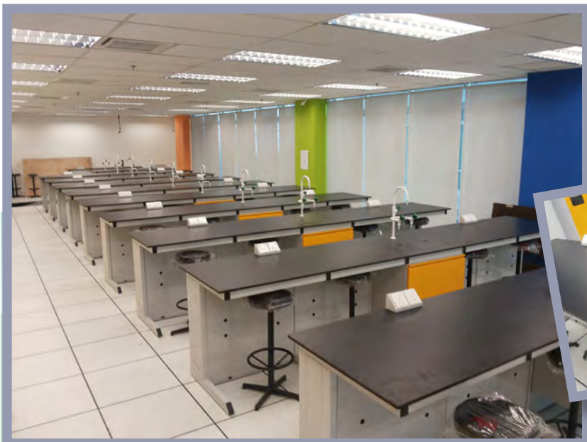
Island bench with one washing area. Sink opening is covered with re-movable worktop material for dry lab usage
